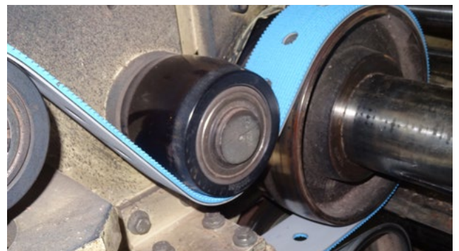
Polyamide foil tensile member offer high flexibility and edge stability.
