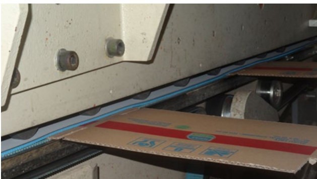
Excellent grip of carton and increased output thanks to wear resistant XNBR Elastomer cover with P6 structure.
