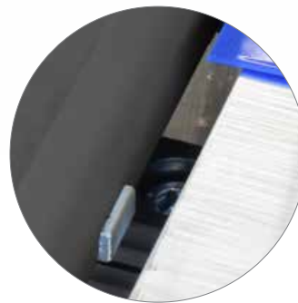
Stopper for precise, repeatable welding
